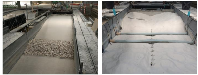
Fig. 5 The small scale 2D-physical model at the Coastal Engineering Laboratory of Politecnico di Bari, Italy. Upper panel: submerged sill, Bottom panel: the drainage system.
