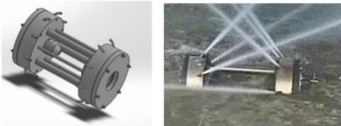
Figure 2: The ejector technology (Bianchni et al., 2014): 3D design (left) and laboratory tests (right).
