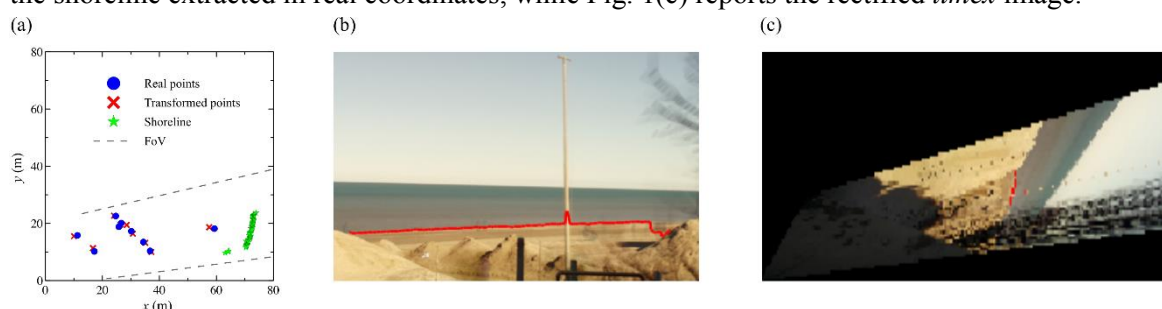
Figure 1. (a) Transformation from the pixel coordinate system to a local reference system in m. (b) Timex with the shoreline (in red) automatically detected. (c) Rectified timex image.
