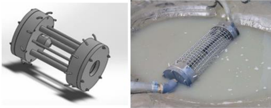
Figure 2. The ejector technology (Bianchni et al., 2014): 3D design (left) and laboratory tests (right).
