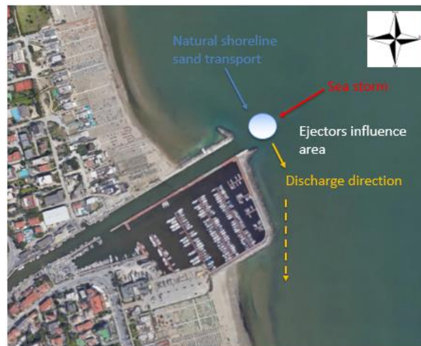
Figure 3. The harbor of Cervia. As shown, ejector restore the natural movement of sediments from North to South that it is currently impeded by the port infrastructure.
