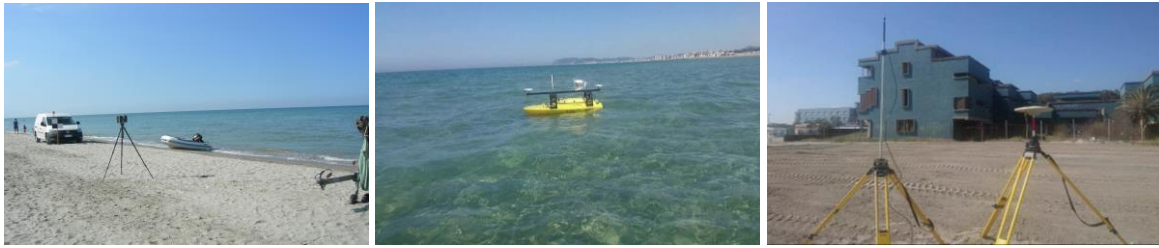
Figure 1. a) TSL survey; b) Autonomous Surface Vehicle for multibeam bathymetric surveys; c) RTK-GPS system used for positioning.
